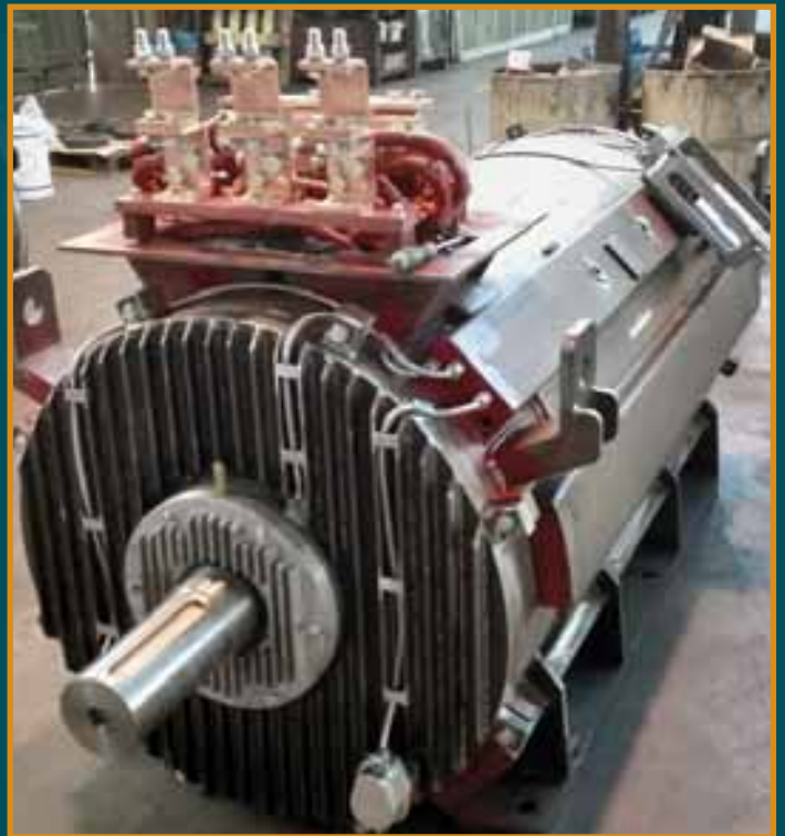
Water jacket motor during final assembly in Beverate di Brivio, LC - Italy
